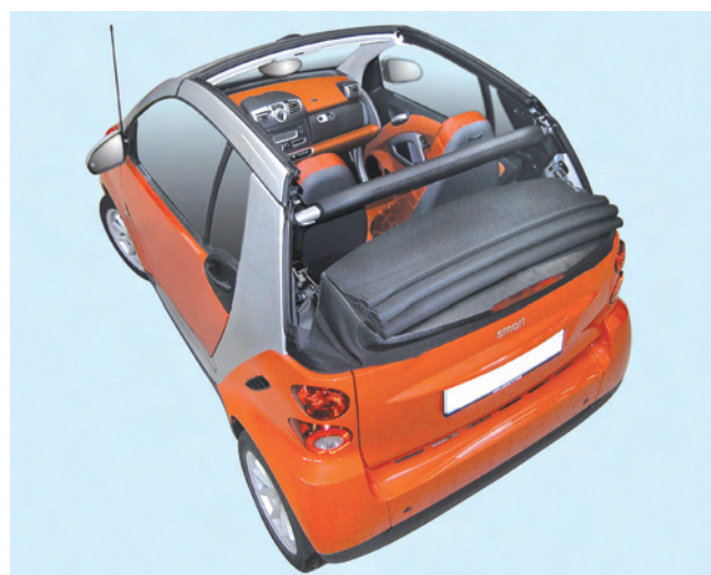
Vehicle with fully electric Tritop fabric soft top
